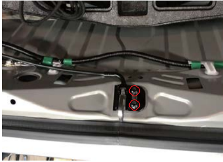
17. Install the electric suction lock assembly, adjust the up and down to the best position, tighten the screws
