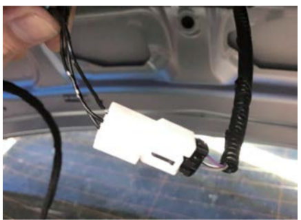
25. The red signal cable is connected to the original lock purple color block plug, orange connect to gray, or with the provided non-breaking wire adapter wiring
