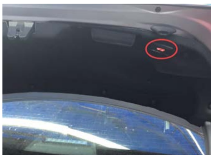
30. The tailgate closing button is fixed on the right side of the tail cover
