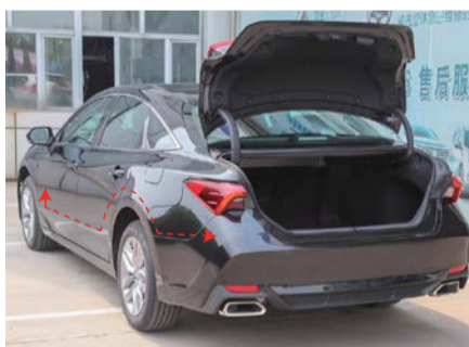
26. The positive pole of the power supply goes along the left side of the trunk to the underside of the driving instrument.
