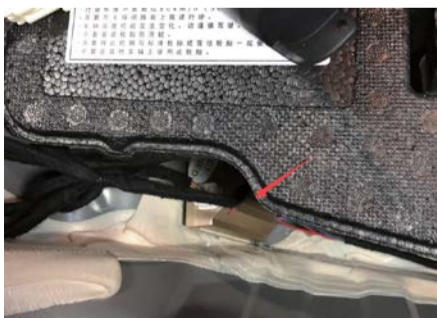
29. Controller fixed on the left side of the trunk
