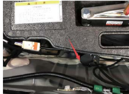
19. Electric suction lock motor is fixed with adhesive
