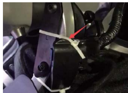
31. After installation, please check the cable tie strap is tied to the plastic case.
