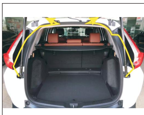
7. Line poles from the lamp go through the waterproof glue plug door cover plate in line to end
