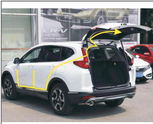
13. Leave the power cord, Central Line through the original car waterproof glue plug door line to end
