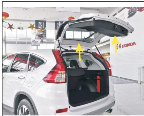
1. Remove the original car plate and the original car poles, someone must be in the middle note down when the poles to hold the car door
