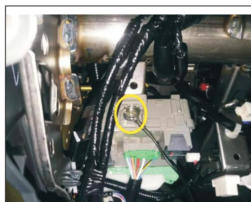
9. In the main driving power on the left side, find the grounding screw, connecting the ground wire
