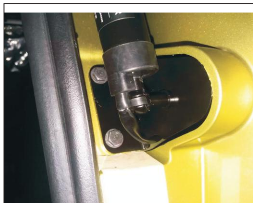
4. Remove the original car right bracket, installation special bracket at the lower right, with the original screw fixation
