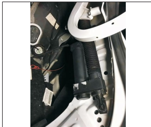
9. Strut installation is complete
