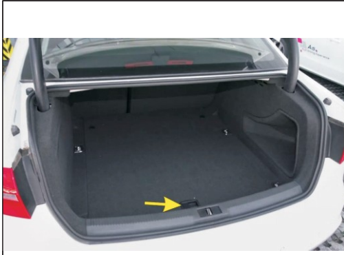
1. According to the arrow position to take out the trunk base plate
