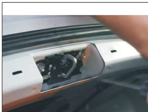
12. Remove the original lock button as shown in figure, the installation our electric lock
