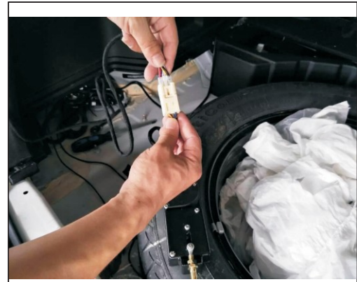
16. The electrical socket to plug in the suction line socket
