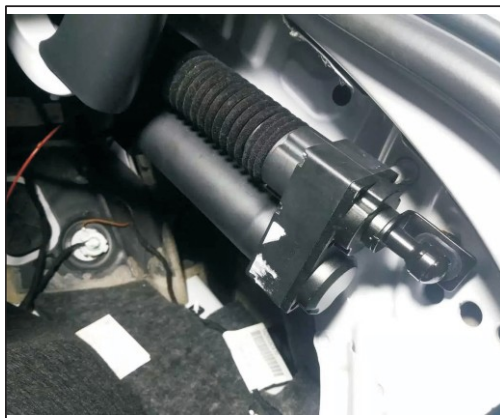
8. Installed as shown our ball head and brace
